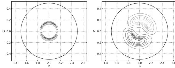
**Fig. 1.**  $V_\phi$  contours of linear tearing mode. Characteristic  $m = 1$  resistive tearing mode (left) is significantly altered by FLR effects (right). Dark circle at  $r = .5\text{m}$  is simulation boundary.
