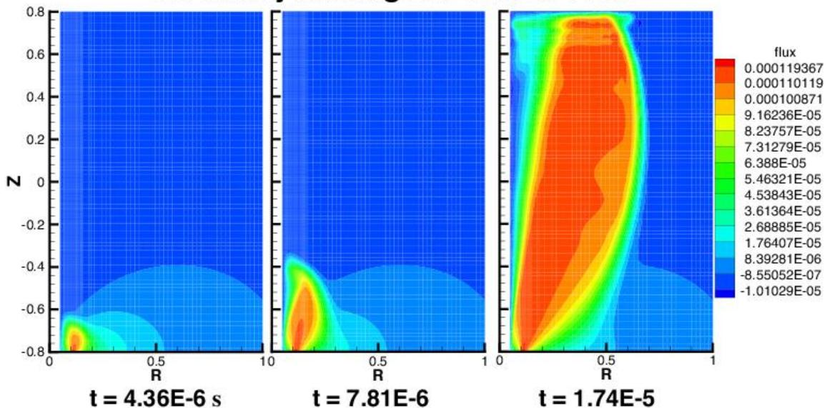
Figure TFT.1. Contours of toroidally averaged poloidal flux from a simulation of coaxial injection in small-aspect-ratio tori. The three frames show three different times during the evolution.
