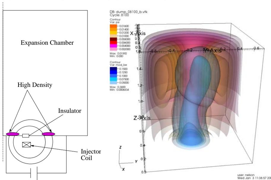
Left: sketch of calculation setup (“Bellan’s box”); Right: toroidally-averaged flux surfaces (brownish) and mod-**B** surfaces in kink-mode (bluish).
