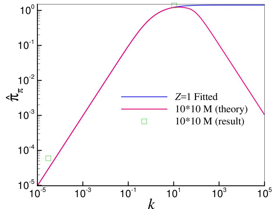
Parallel heat flow and viscosity responding to the temperature and flow velocity gradients, respectively. The NIMROD results (squares) are compared to the analytical integral closures.
